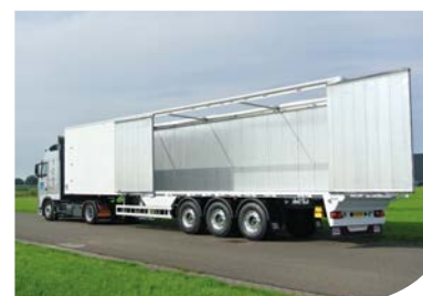
Self-supporting construction with side doors
